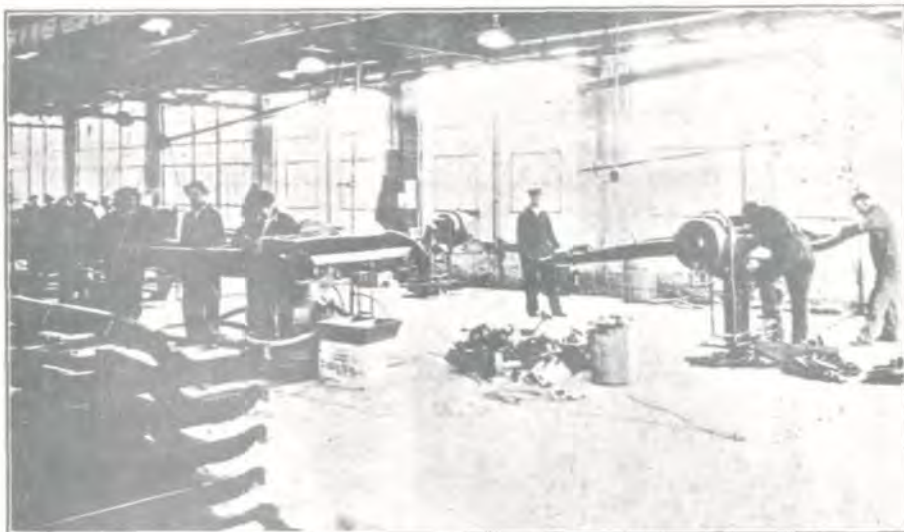
Mechanical hoists and riveting machines speed up production
