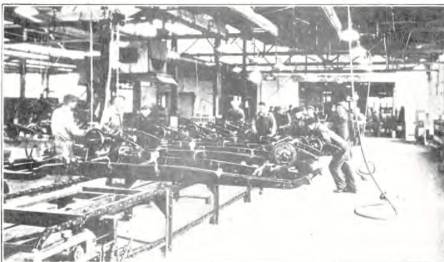
Note how the frames travel on this line—crosswise and upside down
